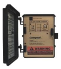
Select a convenient location to mount the Control, making sure that the location is greater than 5 feet from the Pool or Spa and no further than 15 feet from the Solar Valve. Wall-mount the Control, using appropriate screws through the three external mounting points located on the side of the enclosure.
