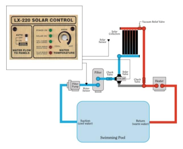
Plumb system in accordance with recommended hydraulic schematic.
