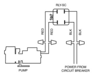
If a solar booster pump is being used, install a Relay kit (model RLY-SC) at the Solar Control in accordance with instructions provided.
