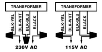
The high voltage wiring section is located behind the service panel in the lower right side compartment of the Solar Control. Holes are provided on bottom of enclosure for conduit mounting. The Solar Control can be connected either to 115VAC or 230VAC. The Solar Control should be wired so that it gets continuous power (connect to Line-Side of Time Clock or directly to sub-panel).
