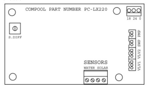
It is possible to control a maximum of two Valve Actuators. Plug the second Valve Actuator into VLV2 socket.
