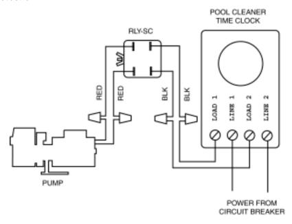
Recommended for use in pool systems which utilize a "booster pump" pool cleaner. This feature automatically turns off the pool cleaner pump for a few minutes whenever solar is initiated. This will protect the pump from damage caused by air in the solar panels at system start-up.
